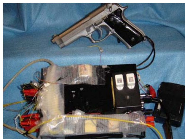
REAL THING—The fourth generation of smart gun now being used in the test firings is shown above with its digital signal processor box. The box takes information relayed to it from the shooter's grip and compares that data to stored information. Eventually when smart gun is manufactured and ready for users, it will contain inside the gun handle a miniature version of the processor box shown above.
