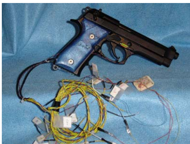
REPLICA GUN—Researchers used this fourth-generation replica of smart gun for demonstration purposes. The attached wires would be used to transfer data from the sensors on the gun grips to the digital signals on a processor box. The processor box is not shown.
