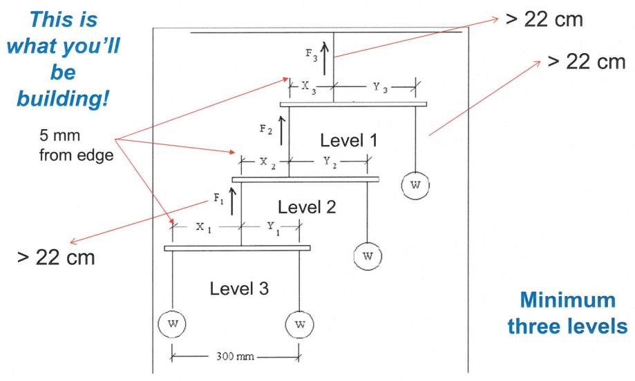
Rods of level 3 and 2 are tied to rods of level 2 and 1 respectively, at a distance of 5 mm from the edge of the lower level rod
