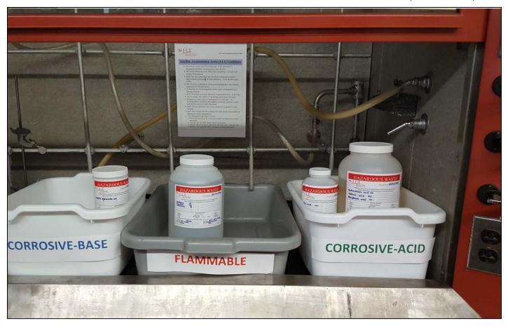
In this example the SAA has been set up to accommodate 3 separate waste streams – flammable, acid, and base.
