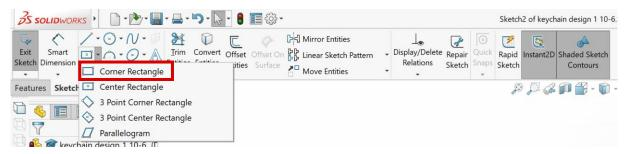
e. Draw a rectangle anywhere on the face of the keychain. We will constrain and dimension this rectangle to ensure it is centered
