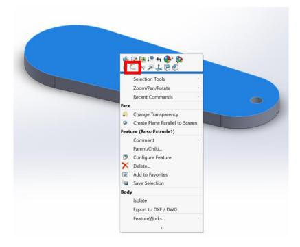
b. Press ctrl+8 to ensure the sketch view is normal to the sketching surface
