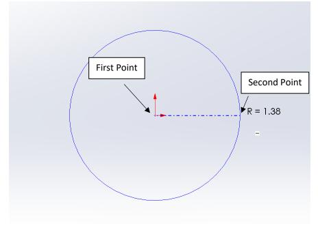
4. Use the "Smart Dimension" tool to set the diameter of the circle just drawn
