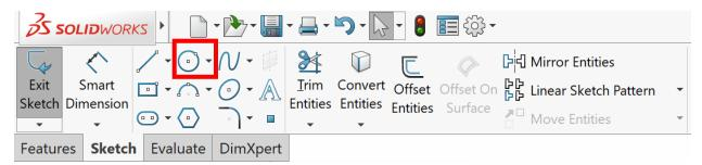
b. Select the origin as the center of the circle first by clicking on the origin, then select a point on the circle's circumference that will determine its diameter
