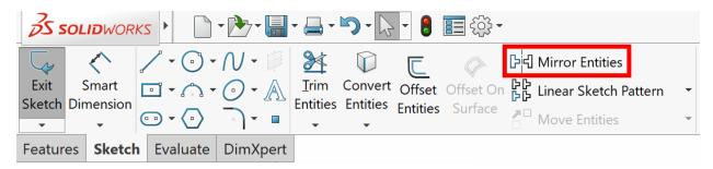
k. First select the line we would like to mirror (the line we just constrained) to mark it as an entity to mirror
