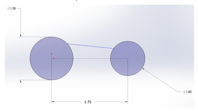
e. Hold the "control" key on your keyboard and select the line just drawn **and** the left circle. This will open the "Properties" pane on the left side of the screen. Here, we can add "constraints" to our drawing
