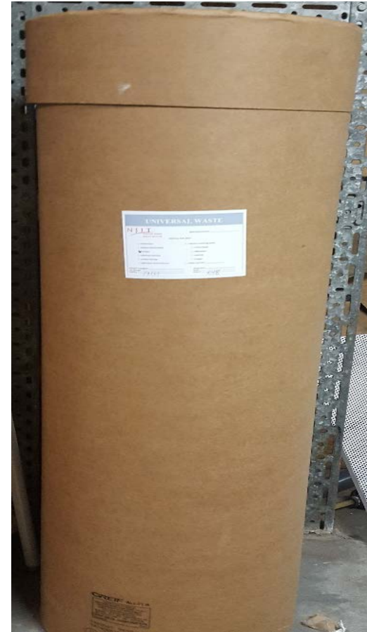
Light tubes properly packaged and labeled as Universal Waste
