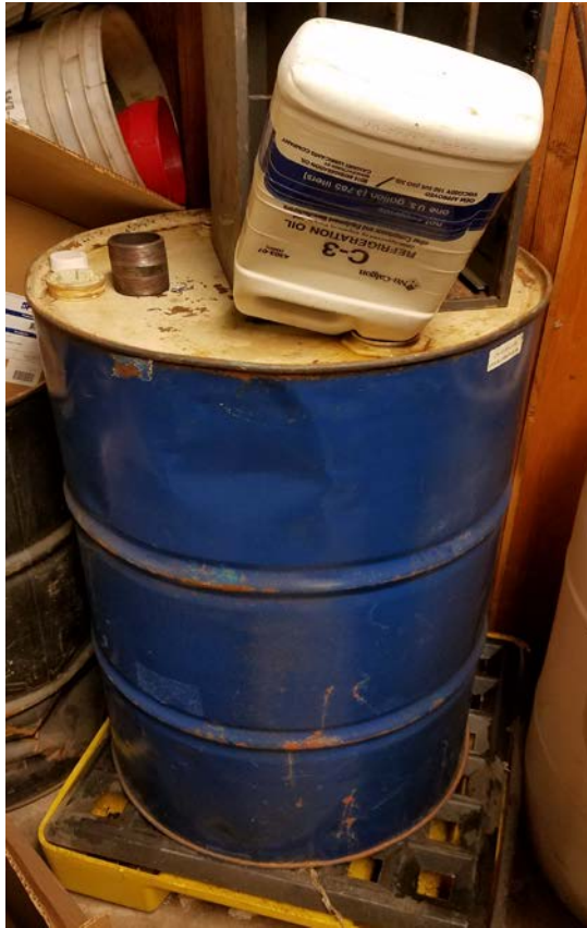
Unlabeled and Unsealed Drum of Used Oil
